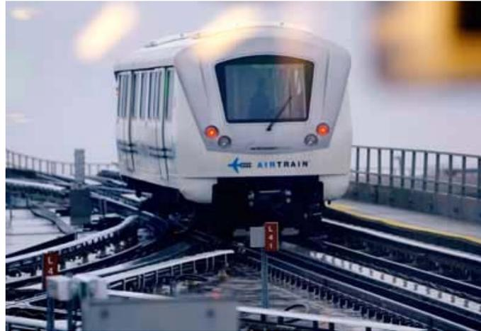
The recently opened AirTrain JFK is a 24 hour driver-less advanced rapid transit system operating on an 8.1 mile, predominately elevated, dual guideway. It connects the 8 JFK Airport terminals to the Long Island Rail Road at Jamaica station, and to the Howard Beach subway station. The light rail vehicles provided by Bombardier are 32 new Mark II cars for which Trak Com designed and provided the onboard communications system.
